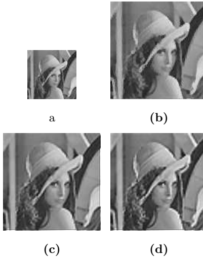
Fig. 3. Comparison of proposed method with alias-free interpolation method [20] approach for 2\times zoom : (a) Input LR image, (b) Image interpolated using alias-free Interpolation method [20], (c) SR using modified TV based approach using only 2 bands, (d) reconstruction using 4 bands.
